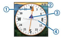
The course pointer ① indicates your relationship to the course line leading to the destination. The course deviation indicator (CDI) ③ provides the indication of drift (right or left) from the course. The scale ② refers to the distance between dots ④ on the course deviation indicator, which tell you how far off course you are.
