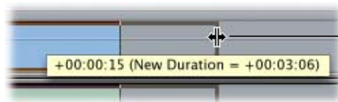
When you use the Selection tool to adjust a clip’s edit point, the icon changes to indicate it can be used for trimming.
