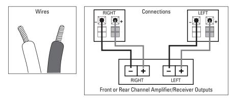
Speakers and electronics terminals have corresponding (+) and (-) terminals. It is important to connect both speakers identically: (+) on the speaker to (+) on the amplifier and (-) on the speaker to (-) on th amplifier. Wiring 'out of phase' results in thin sound, weak bass and a poor stereo image.
