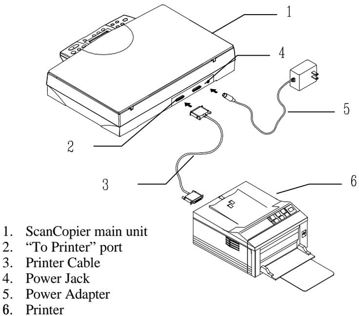
**Figure 2-2 Connect ScanCopier to a printer**
