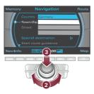
3 Press the rotary push-button to confirm.
