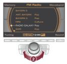
Press the rotary pushbutton. The next free position in the memory list will be highlighted.
