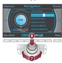
8 Press the rotary pushbutton to confirm.
