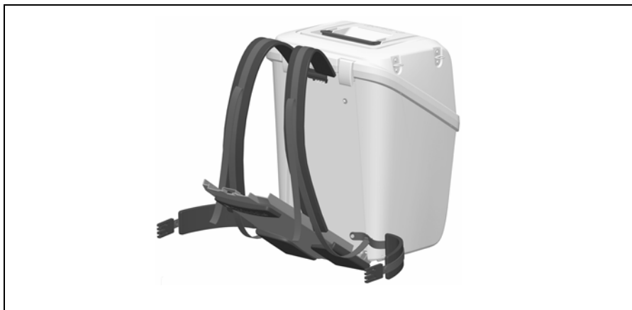
Figure 2.3 Fitting the carrying straps
