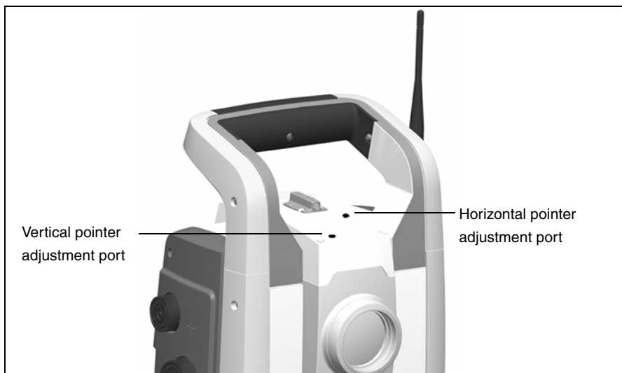
Figure 4.33 Laser pointer adjustment ports
