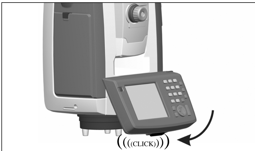
Figure 4.40 Attaching the Trimble CU
