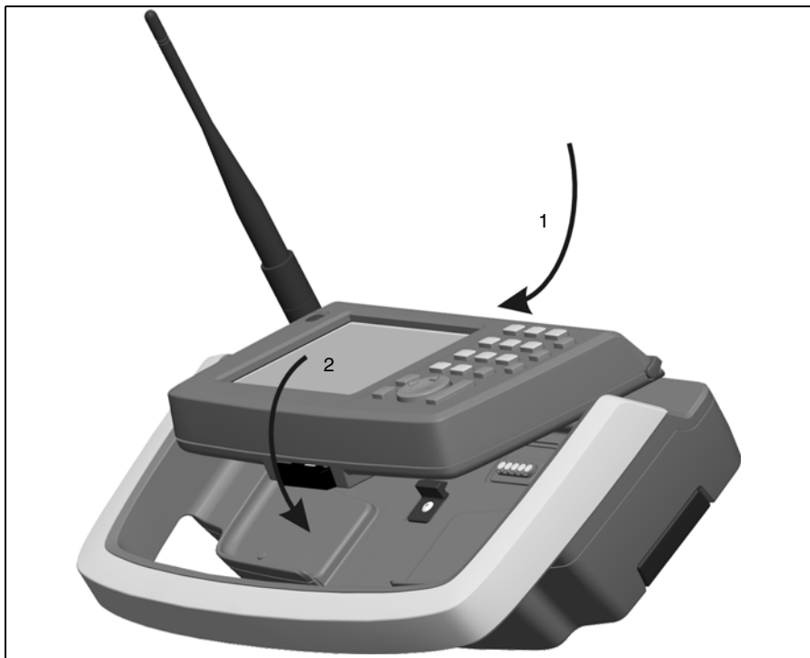
Figure 7.78 Attach Trimble CU to Trimble Robotic Holder
