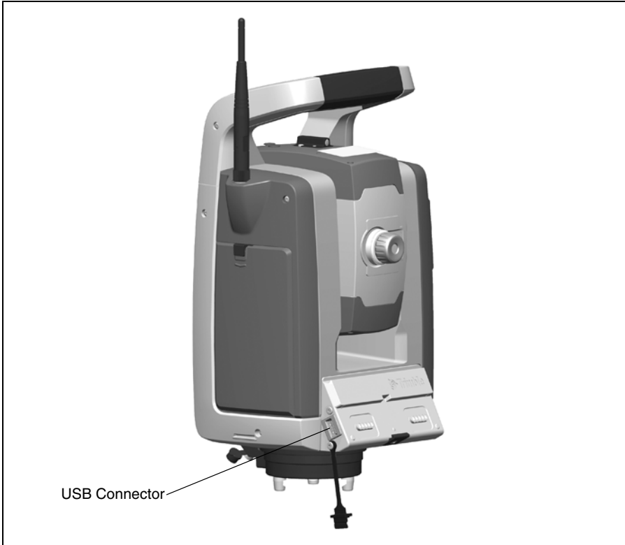
Figure 6.60 The USB Connector.
