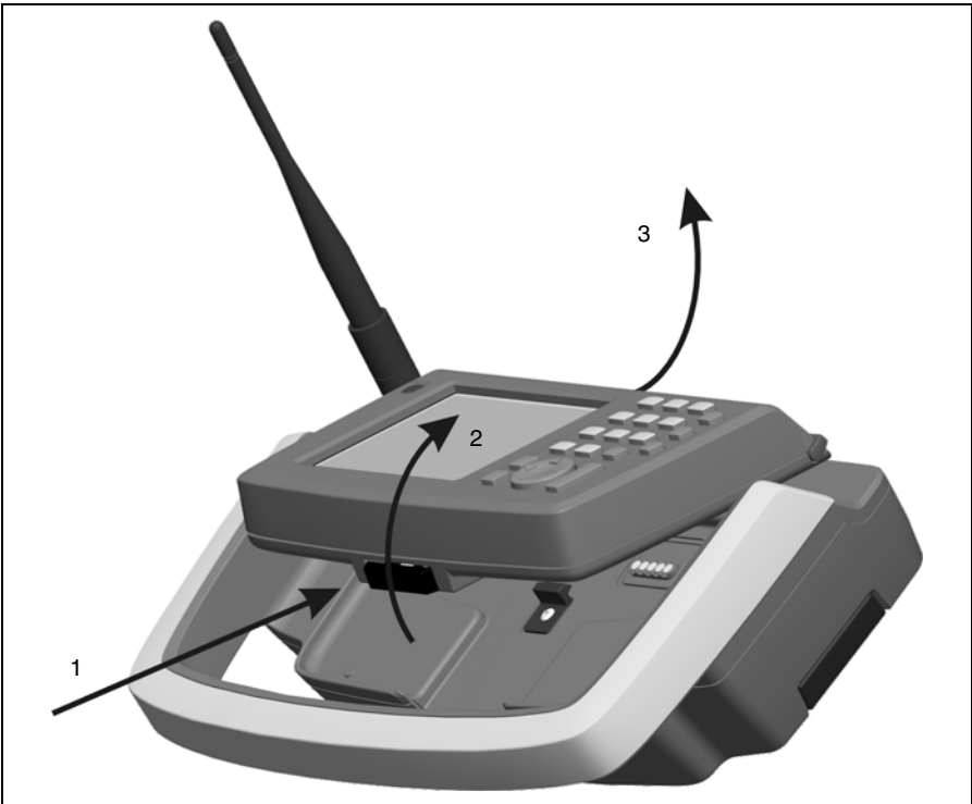
Figure 7.79 Detach Trimble CU from Trimble Robotic Holder
