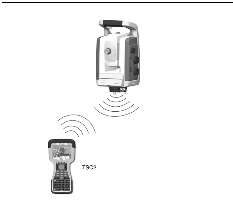
Figure 4.44 TSC2 connected to the Trimble S Series Total Station with Bluetooth wireless technology for servo and Autolock measurements.
