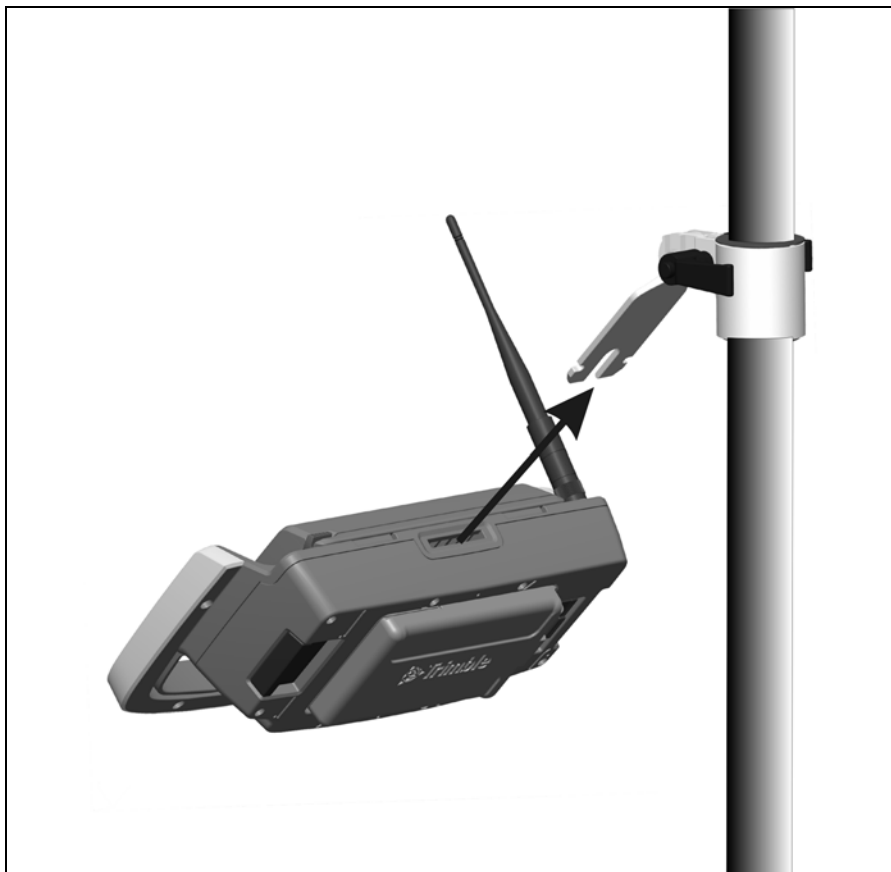
Figure 7.80 Attaching the Trimble Robotic Holder to the standard rod adapter
