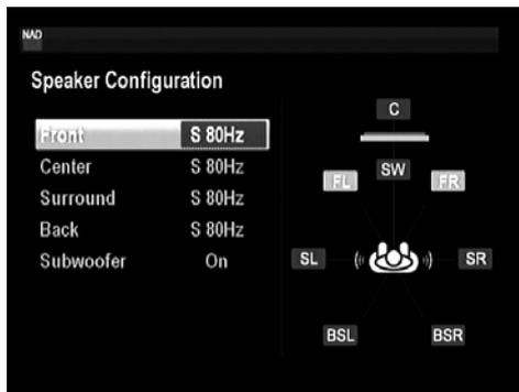
Every surround-sound system requires “bass-management” to direct low-frequency content from any or all channels to the speakers best able to reproduce it. For this function to operate correctly, it is important that you correctly identify your speakers’ capabilities. We use the terms “S” (Small), “Large” and “Off”, but note that physical size may be irrelevant.
