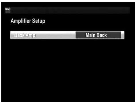
If the surround back speakers are not used in the main zone, their surround back amplifier channels could be assigned for Main Back or Zone 2.
