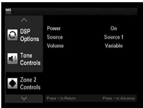
The Zone feature allows one to simultaneously listen to an active Source of the T 747 that is different from the currently selected Source.
