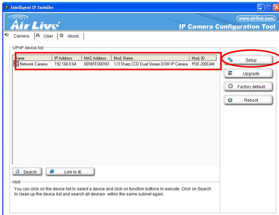
7. Follows setup instruction to change the IP address of the IP Camera.
