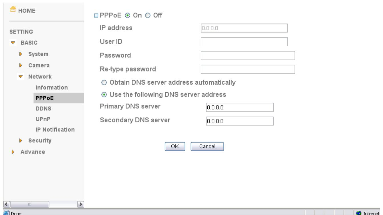
**IP address** : The IP address obtained at the PPPoE connecting with network.
