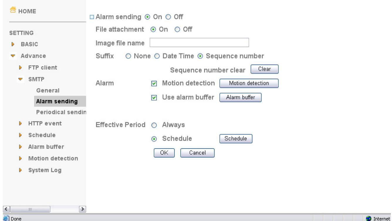
**Alarm sending :** Select **On** to set to send mail with connection to the alarm detection.
