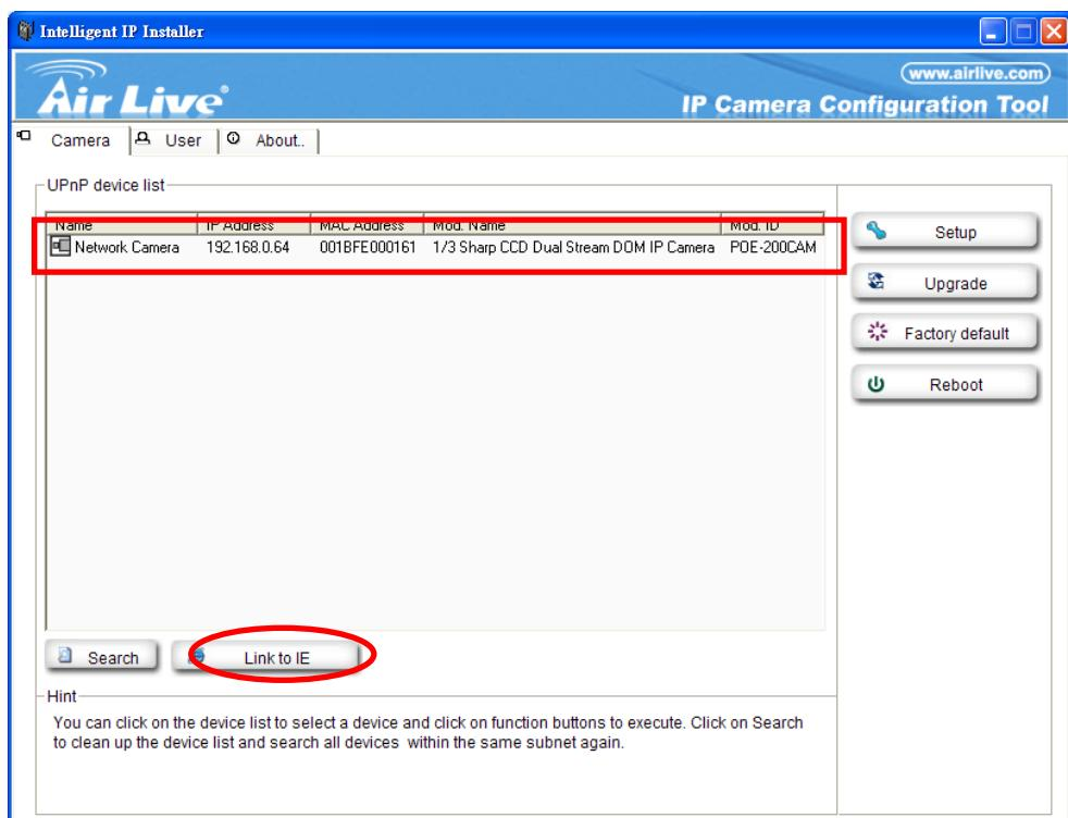
6. If the IP is not in your IP segment, select the founded IP Camera and click "Setup".
