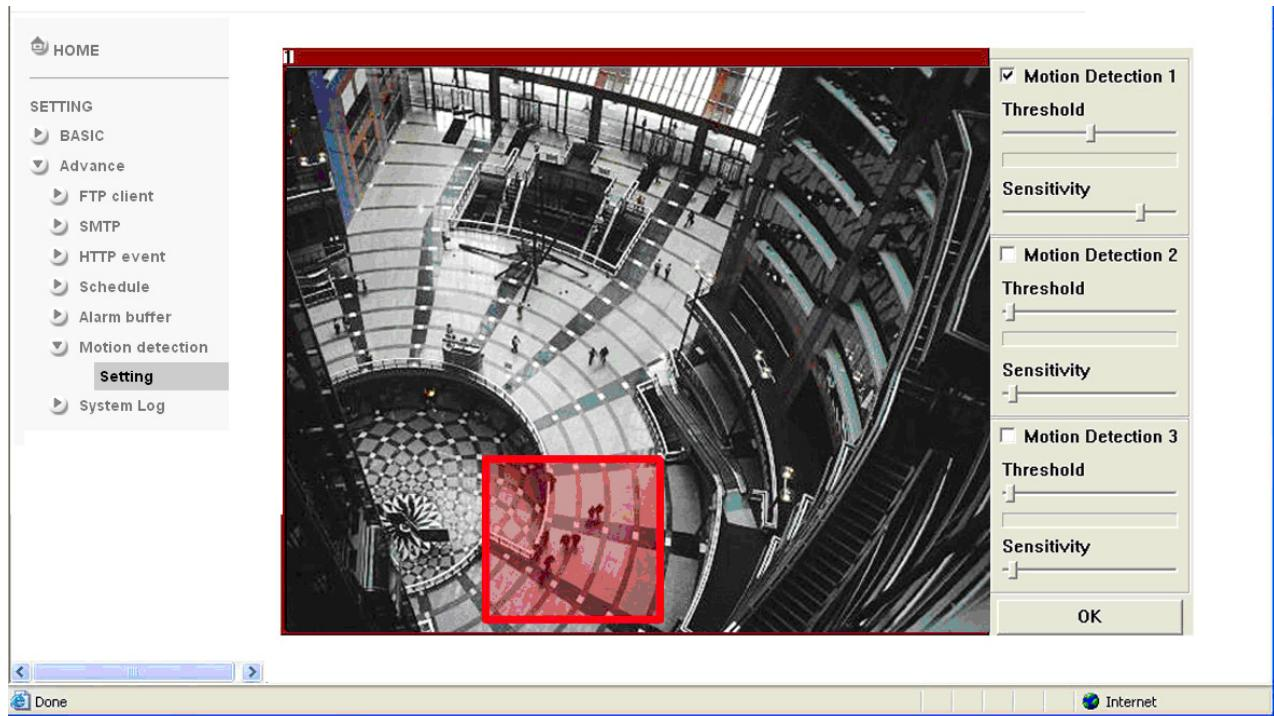
Click it **On** when you use the Motion Detection function and detecting zone appears for adjusting and moving. The common setting options are displayed below. If you do not wish to use the Motion Detection function, click it **Off** and press **OK**.
