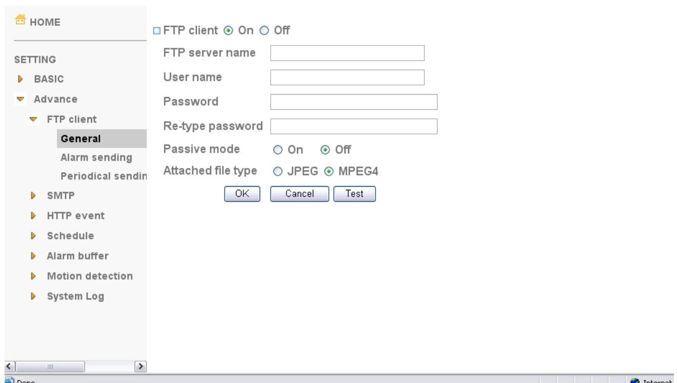
**FTP client function** : To activate the FTP client function, select **On**. The FTP client setting page appears. When you do not wish to use the FTP client function, select **Off**.
