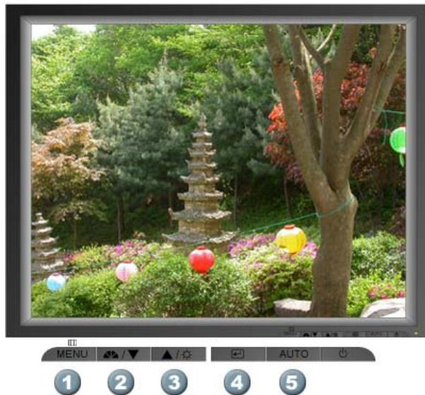
1. [MENU] Use this button to open the on-screen menu and exit from the menu screen or close screen adjustment menu.
