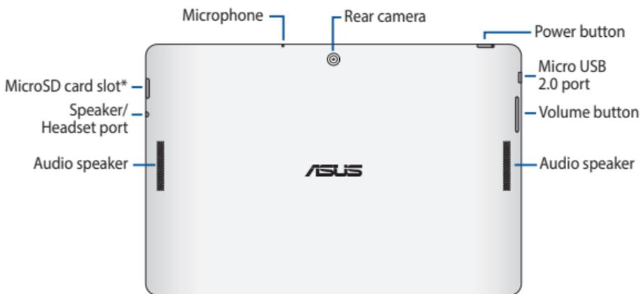
\* The microSD card slot supports microSD, microSDHC, and microSDXC card formats.
