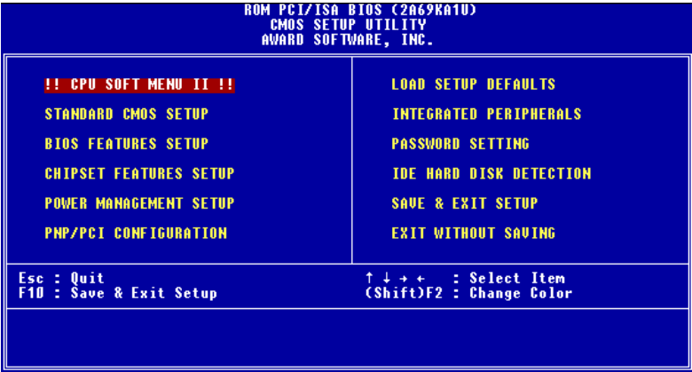
Figure 3-1. CMOS Setup Utility
