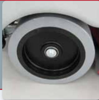
New polyurethane drive and rear tyres: outstanding traction, either on dry or wet floors, non marking, high wear resistance
