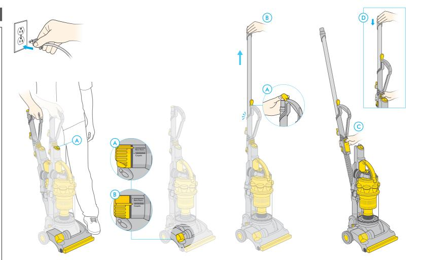
After plugging machine into electric outlet, press on/off button **A**, push cleaner head down with foot and pull handle towards you.
