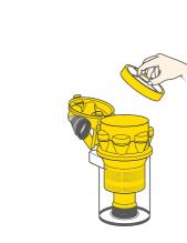
Press cyclone release button **A** to release cyclone pack.
