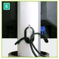
**Cable Fix Ring:**When connecting the cable is finished fix the cables to the Cable Fix Ring.
