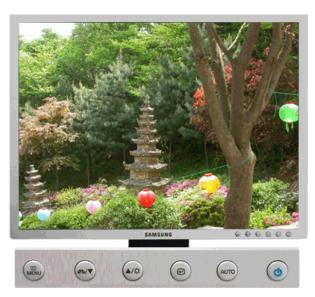
Menu Description **\ Brightness** When OSD is not on the screen, push the button to adjust brightness.
