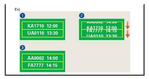
The best way to protect your monitor from Image retention is to set your PC or System to operate a Screen Saver program when you are not using it.
