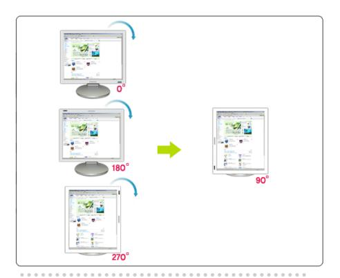
Rotate to 180 : Display will get rotated to 180 degree from the current angle of rotation.
