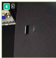
Kensington Lock: The Kensington lock is a device used to physically fix the system when using it in a public place. (The locking device has to be purchased separately.)
