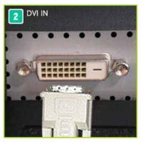
**DVI IN port**: Connect the DVI Cable to the DVI IN port on the back of your monitor. (SOURCE: Digital)
