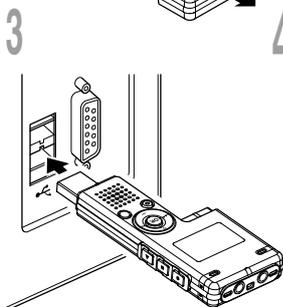
**3 Connect the recorder's USB terminal to a PC USB port or USB hub.**
