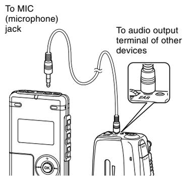
The sound can be recorded when connecting to the audio output terminal (earphone jack) of the other device, and the microphone jack of the recorder with the connecting cord (optional KA333)<sup>(P.84)</sup> for dubbing.
