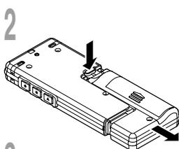
**2 Detach the battery compartment pressing the **RELEASE** button of the rear side.**
