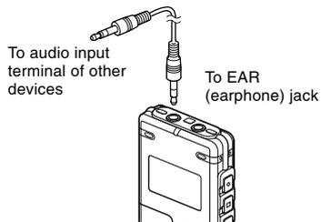
The sound of this recorder can be recorded to other devices when connected to the audio input terminal (microphone jack) of other devices and the earphone jack of this recorder, with the connecting cord (optional KA333) for dubbing.
