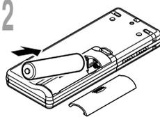
2 Insert size-AAA alkaline battery, observing the correct polarity.
