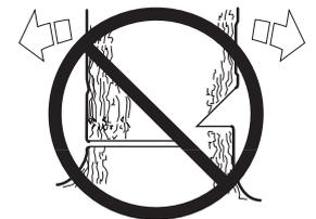
When the felling cut and directional cut are complete the tree should start to fall under its own weight or with the aid of a FELLING WEDGE.
