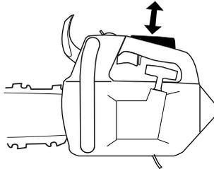
3 Check that the throttle control and throttle lock move freely and that the return springs work properly.
