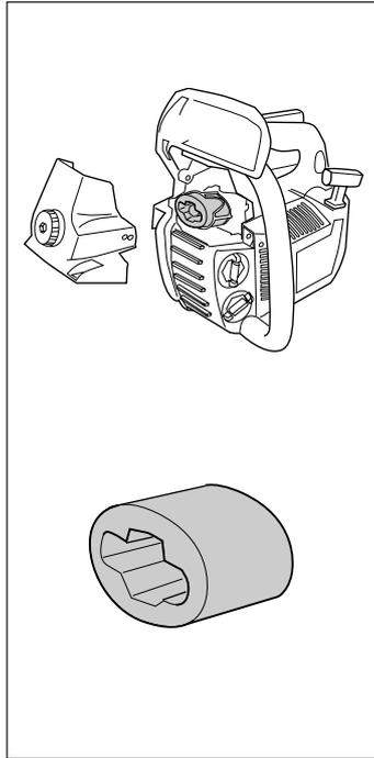
An air filter, which is used for some time, cannot be cleaned completely. Therefore it must be replaced by a new one, with regular intervals.
