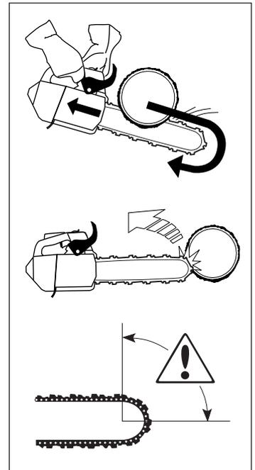
Unless the user resists this pushing force there is a risk that the saw will move so far backwards that only the kickback zone of the bar is in contact with the tree. This will cause kickback.
