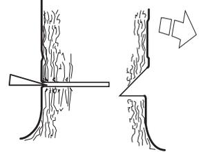
Finish the FELLING CUT parallel with the DIRECTIONAL CUT LINE so that the distance between them is at least 1/10 of the trunk diameter. The uncut section of the trunk is called the HINGE.
