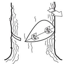
All control over the felling direction is lost if the HINGE is too narrow or if the directional cut and felling cut are badly placed.
