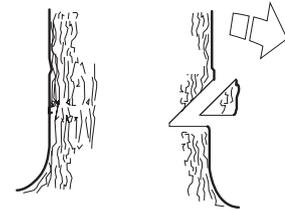
The directional cut should run 1/4 of the diameter through the trunk and the angle between the TOP CUT and BOTTOM CUT should be 45°.
