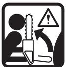
Tip contact may cause the guide bar to move suddenly upward and backward, which may cause serious injury.
