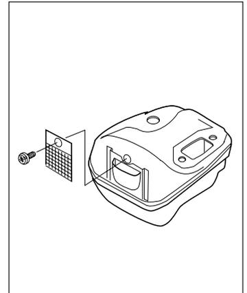
With this type of muffler it is very important that you follow the instructions on checking, maintaining and servicing your saw (see the section on "Inspecting, maintaining and servicing chain saw safety equipment").
