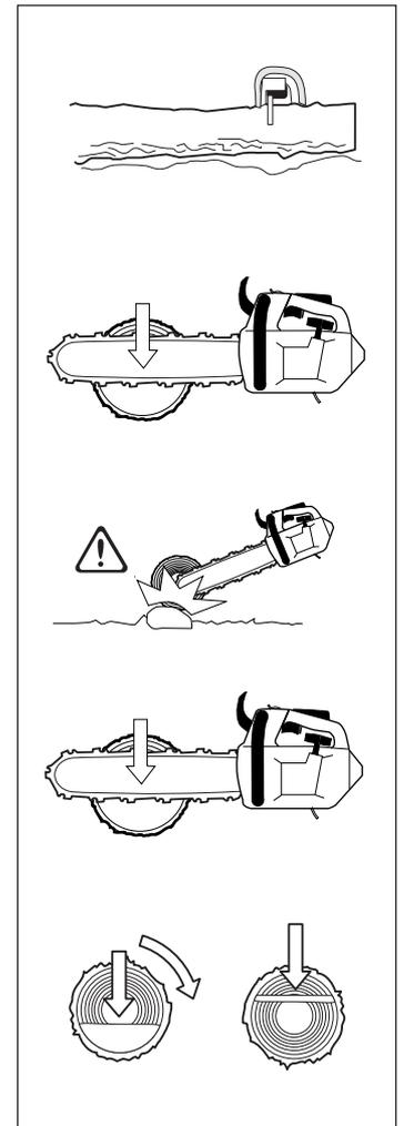
Cut all the way through the log from above. Try not to touch the ground as you finish the cut. Maintain full throttle but be prepared in case the chain snatches.
