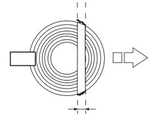
The HINGE act as hinges that control the felling direction of the falling tree.
