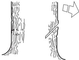
Next make the BOTTOM CUT so that it finishes at the end of the TOP CUT.
