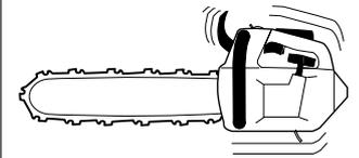
Make sure the vibration damping units are securely attached to the engine unit and handles.
