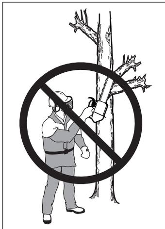
If you have to saw tree limbs or the like that are above shoulder height, stand on a work platform or a work stand. Never use the saw while standing on a ladder.
