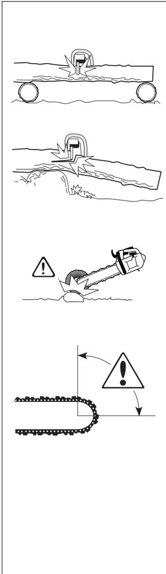
Two factors decide whether the chain will jam or the log will split. The first is how the log is supported and the second is whether it is in tension.
