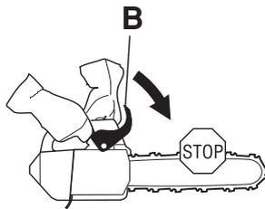
This movement activates a spring-loaded mechanism that tightens the Brake Band (C) around the engine drive system (D) (Clutch Drum).
