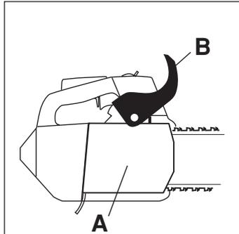
The brake is applied when the front hand guard (B) is pushed forwards.
