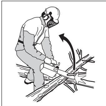
4 Never use the saw above shoulder height and do not cut with the tip of the bar.
