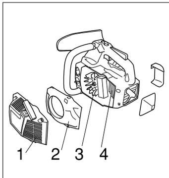
Clean the cooling system with a brush once a week, more often in demanding conditions. **A dirty or blocked cooling system results in the saw overheating which causes damage to piston and cylinder.**
