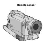
When using the remote control, be sure to point it at the remote sensor. The transmitted beam's approximate effective distance for indoor use is 5m.
