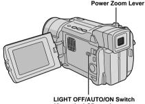
LIGHT OFF/AUTO/ON Switch (Open the LCD monitor to access this switch.)
