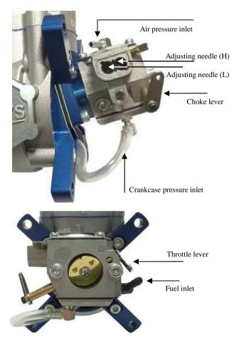
Caution! Never tighten the adjusting needles with too much strength. This may cause damage of the needles. If the needles are damaged this way it is no longer possible to adjust the carburetor and it is necessary to exchange it for a new one.
