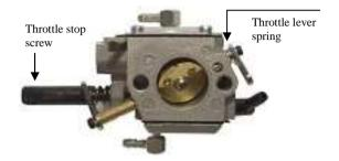
If the throttle pull rod is not equipped with flexible element it is recommended NOT to put off the throttle valve spring. Otherwise the vibrations of the engine can cause excessive wear of the throttle valve shafting and with this deteriorate the carburetor function.
