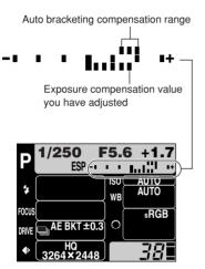
If the selected range is beyond the scale of the exposure level indicator, only the part within the scale is displayed.
