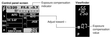
The exposure compensation indicator disappears if the exposure is compensated by 0.
