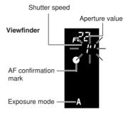
Underexposed when the shutter speed indication is blinking. Decrease the aperture value (F-number).
