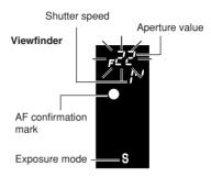
If the aperture value indication at the maximum value is blinking, the correct exposure is not attained (overexposed). Set the shutter speed higher.
