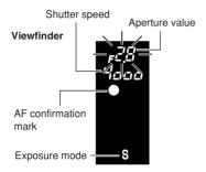
If the aperture value indication at the minimum value is blinking, the correct exposure is not attained (underexposed). Set the shutter speed slower.
