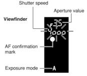
Overexposed when the shutter speed indication is blinking. Increase the aperture value (F-number).
