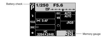
Each time you press the shutter button, the memory gauge lights on the control panel screen, indicating that the picture you have just taken is being recorded onto the card. The memory gauge changes according to how many pictures the camera is processing.
