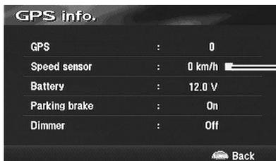
Blinks when the Speed Pulse signal is being input.
