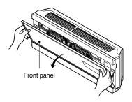
2. Lift up the Front panel. The hook of panel comes off.
