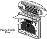
4. Insert the Plasma Filter after perfectly drying in shade.
