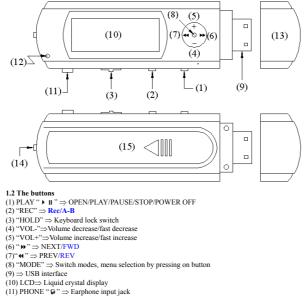
(12) MIC  $\Rightarrow$  Built-in microphone (13)  $\Rightarrow$  USB cover (14)  $\Rightarrow$  Cord hole (15)  $\Rightarrow$  battery cover
