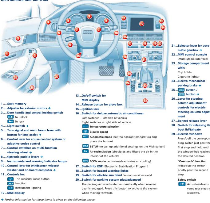
24...Electro-mechanical parking brake -> 25 ... STOP button / ENGINE button -> 26 ... Lever for steering column adjustment/ controls for electric steering column adjust-27 ... Bonnet release lever 28 ... Switch for releasing the boot lid/tailgate 29...Electric windows
