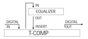
A favorite trick of experienced audio engineers is to employ an equalizer before the signal is piped through a compressor. The MindPrint PARA-Q is the ideal tool for this task—it was designed specifically to work together with the T-COMP. A truly high-quality device, it delivers remarkably musical results.
