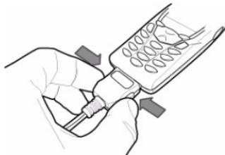
Your telephone is powered by a rechargeable battery. A new battery must be charged for 4 hours at least before being used for the first time. It reaches its optimum capacity after a few cycles of use.
