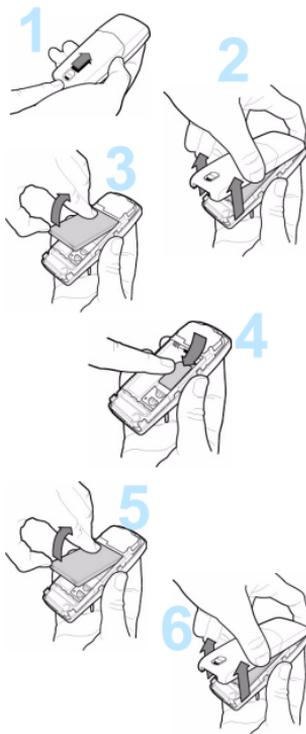
The SIM card is inserted under the telephone's battery. Ensure that the telephone is switched off and the charger disconnected.
