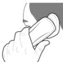
The antenna is embedded in your telephone, under the back cover at the top.
