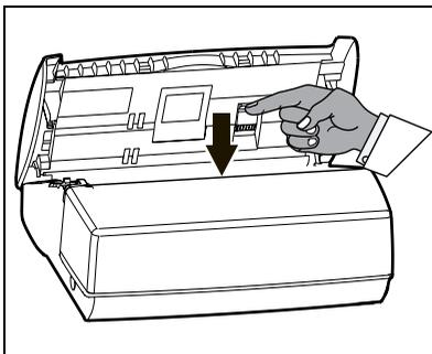
☞ Push downward on the gauge card housing to unlock it: it opens automatically, letting you access the worn gauge card.
