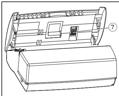
☞ The front cover being open, locate the gauge card housing (7).
