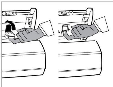
☞ Close the flap of the gauge card housing by rotating it. Once into place, push it upward to block it. Close the cover and replace the handset.
