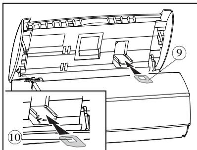
☞ Insert the new gauge card (9) into its housing. Make sure the chip (10) of the gauge card (9) is **upwards, bevelled corner to the top left side**.
