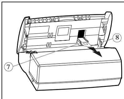
☞ Remove the worn gauge card (8) from its housing.
