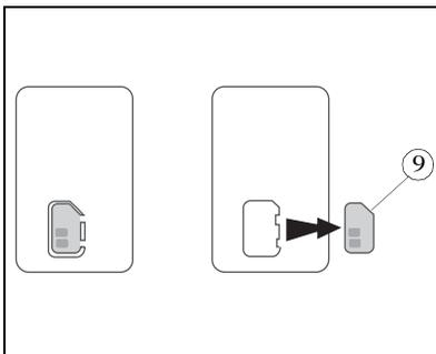
☞ Remove the new (pre-cut) gauge (9) from the ribbon gauge card (8).
