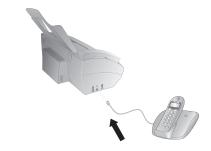
We recommend direct connection to the machine because this allows the fax switch to function optimally and to control the additional devices.
