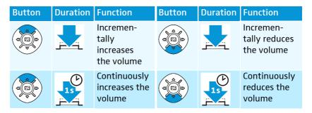
If you press the respective button briefly, the volume is changed incrementally; if you hold down the button, the volume is changed continuously.
