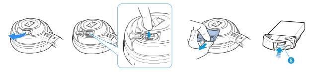
Connect the charging cable 12 to the socket for charging cable 8 on the battery pack.
