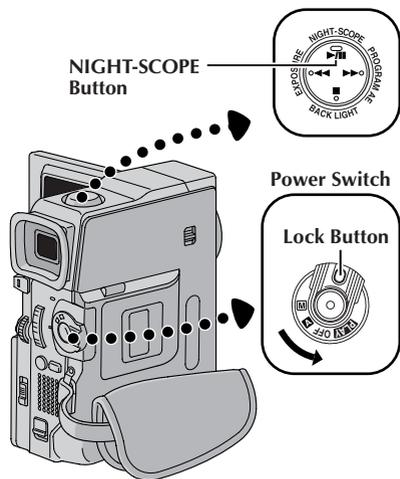
**1** Set the Power Switch to “M” while pressing down the Lock Button located on the Switch. Open the LCD monitor fully or pull out the viewfinder fully.
