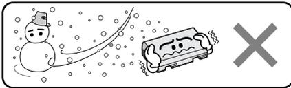
Lithium-ion is vulnerable in colder temperatures.
