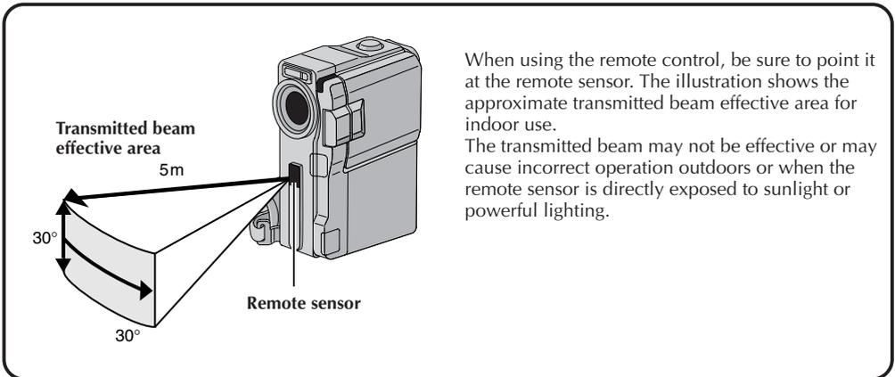
When using the remote control, be sure to point it at the remote sensor. The illustration shows the approximate transmitted beam effective area for indoor use.
