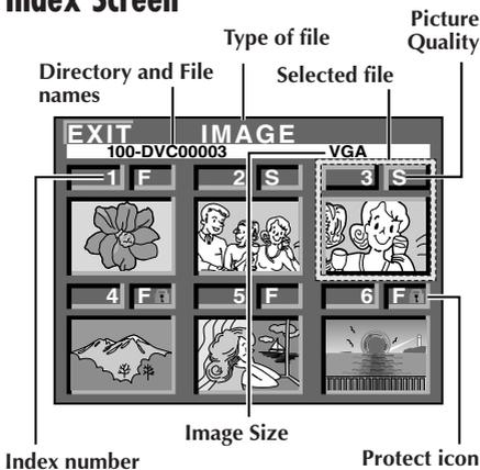
The files you stored can be displayed together with their index information. Convenient for checking files stored beforehand, the Index Screen also shows the Picture Quality, Image Size mode, directory and file names as well as which files are protected against accidental erasure. To display the Index Screen, ☞ pg. 30.
