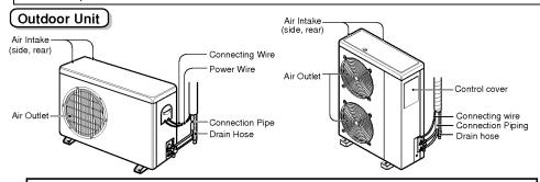
Heat pump model: Cassette Type Air Conditioner for cooling and heating Cooling model: Cassette Type Air Conditioner for cooling
