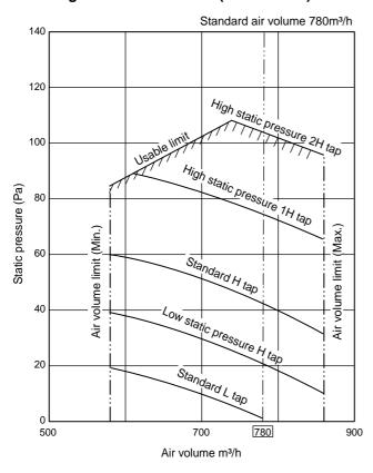
Fig. 3 RAV-SM802BT-E (Round duct)
