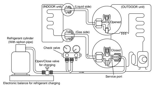
Fig. 7-4-1 Configuration of refrigerant charging
