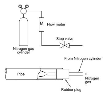
Fig. 7-5-1 Prevention of oxidation during brazing
