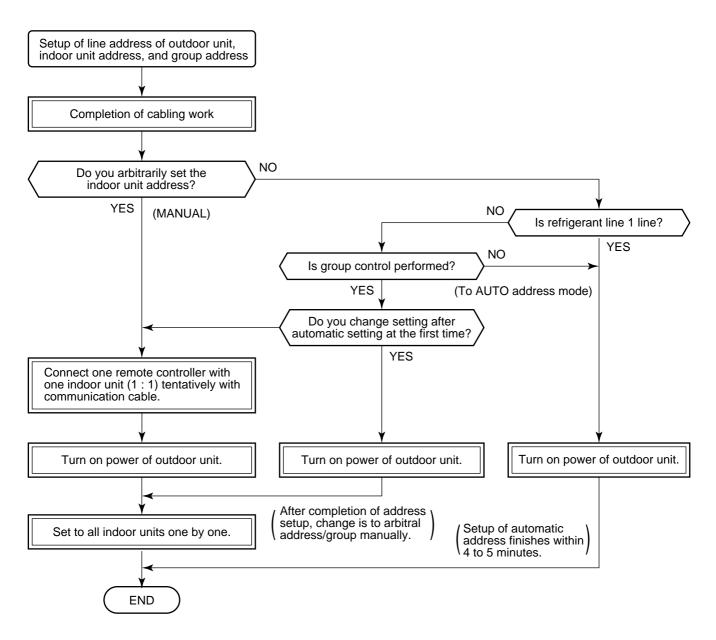
• When the following addresses are not stored in the neutral memory (IC10) on the indoor P.C. board, a test run operation cannot be performed. (Unfixed data at shipment from factory)
