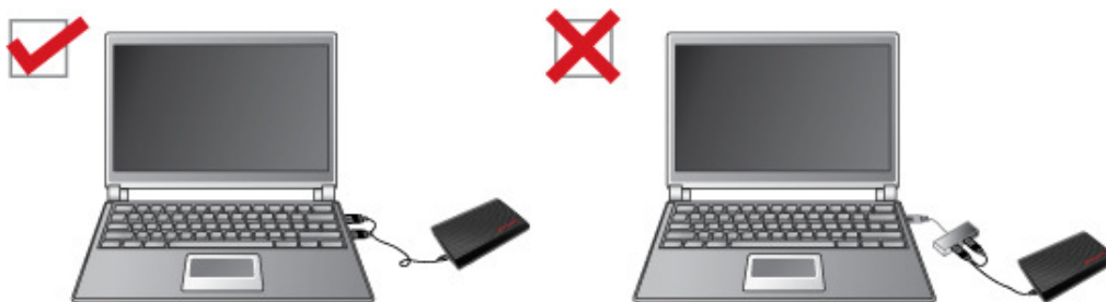
Figure 20: Plug both USB connectors directly to your computer
