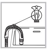
alternatively, rest it on the side of a washbasin of the hose should not be underwater.
