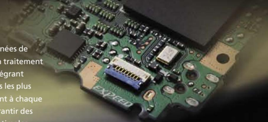
A close-up photograph of a green printed circuit board (PCB) for a Nikon camera. The board is densely packed with various electronic components, including integrated circuits, capacitors, and a blue multi-pin connector. The word "EXPEED" is printed in white on the board near the connector. The background is dark and out of focus.
