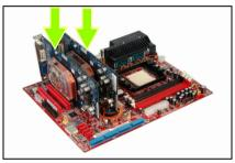
**4.** Insert the two graphics cards into PCIEXP1 and PCIEXP2 slots on the motherboard.
