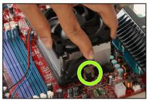
**5.** Place the heatsink and fan assembly onto the retention frame. Match the heatsink clip with the socket mounting lug. Hook the spring clip to the mounting lug.
