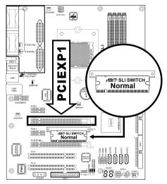
**Normal Mode:** Leave the SLI Switch to its default Normal mode and insert the graphics card into PCIEXP1 slot. The PCIEXP2 slot functions as a PCIE x1 slot under this mode.
