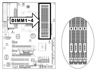
**NOTE:** Usually there is no hardware or BIOS setup requires after adding or removing memory modules, but you will have to clear the CMOS memory first if any memory module related problem occurs.
