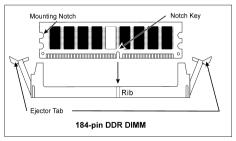
5. To remove the DIMM modules, push the two ejector tabs on the slot outward simultaneously, and then pull out the DIMM module.
