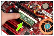
**3.** Slightly push down the switchboard until the retention clip snap into places. Make sure the switchboard is completely inserted into the slot.
