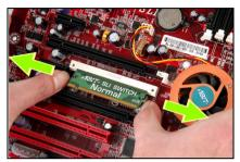
1. Simultaneously push the two retention clips at both ends outward to release the switchboard. Carefully pull the switchboard out of the slot.
