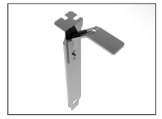
7. The SLI bracket included in the package is used for supporting the SLI bridge connector and the two SLI graphics cards.
