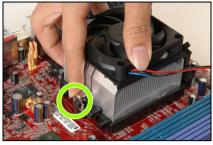
**6.** On the other side, push the retention clip straight down to lock into the plastic lug on the retention frame.
