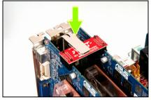
**8.** Insert the SLI bracket into the bracket slot between the graphics cards. Secure the SLI bracket and the graphics cards to the chassis with screws.
