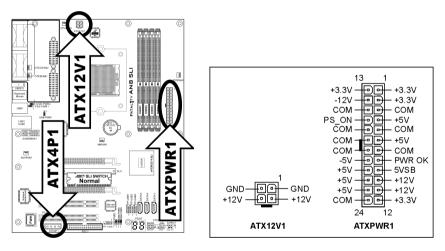
**NOTE:** For a heavily loaded system, a power supply that provides a minimum of 350W and 20A on the +5VDC rail is recommended. To support wake-up features, 2A on the +5VSB rail is required.
