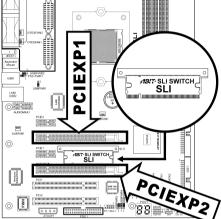
**SLI Mode:** Switch the SLI Switch to SLI Mode and insert the SLI-ready graphics cards into PCIEXP1 and PCIEXP2 slots.
