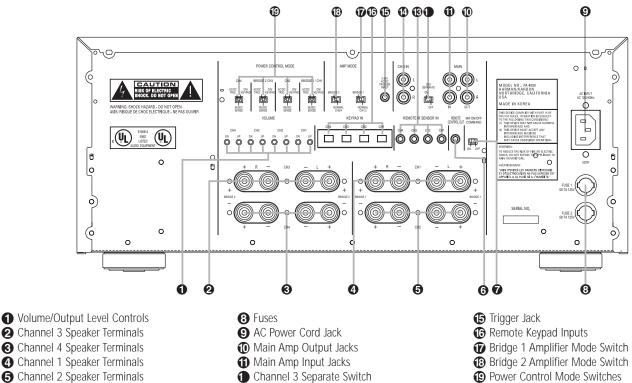
MR On/Off Command Switch **Over the Second Second Press Volume/Output Level Controls:** Press these controls to change the volume level up or down for an individual channel pair in remote room applications. For surround sound applications, use them with the test tone in your receiver or processor to set the output levels. See page 13 for more information.
