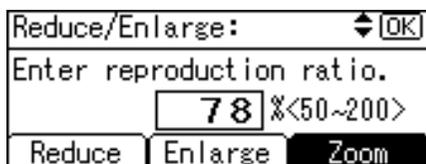
Pressing [▲] or [▼] changes the ratio in increments of 1%. Pressing and holding down the relevant key changes the ratio in increments of 10%.
