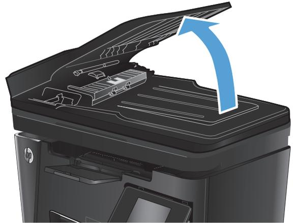
2. Use a moist, lint-free cloth to wipe both pickup rollers and the separation pad to remove dirt.
