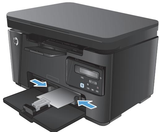
4. Push the paper into the product until it stops, and then push the paper length guide in so the extender tool supports the paper.
