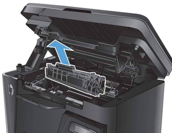
4. Remove any jammed paper from the toner-cartridge area. Use both hands to remove jammed paper to avoid tearing the paper.
