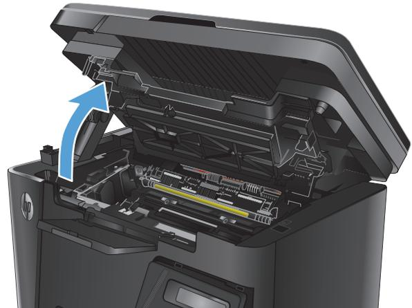
3. Remove any jammed paper from the output bin area. Use both hands to remove jammed paper to avoid tearing the paper.
