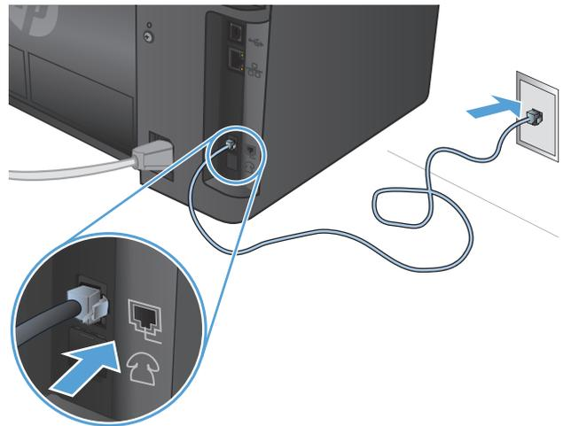
2. (Optional) To connect an answering machine or extension phone, pull down the rubber plug from the telephone port
