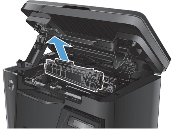
5. Remove any jammed paper visible in the input tray area. Use both hands to remove jammed paper to avoid tearing the paper.
