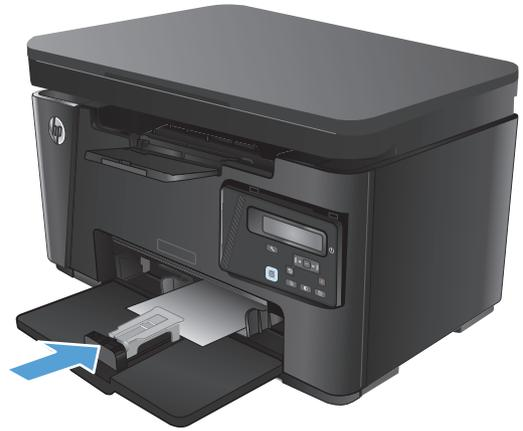
5. When finished printing on short paper, remove the short-paper extender tool from the input tray, and then place it in the storage slot.
