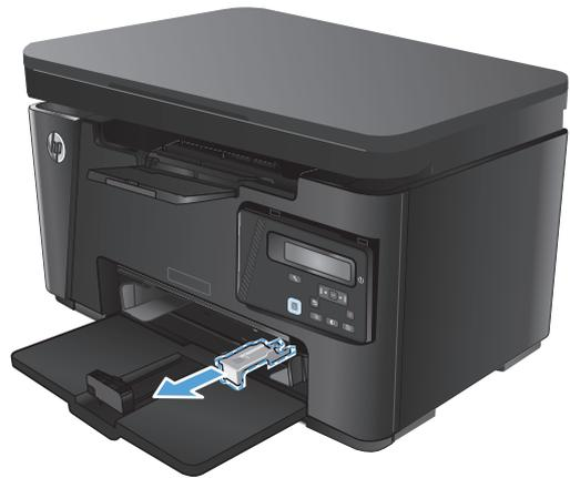
2. Attach the tool to the paper length guide on the input tray.
