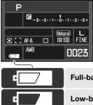
This camera is equipped with an automatic battery-condition indicator. When the camera is on, the indicator appears on the monitor. The indicator changes from white to red when battery power is low. If the monitor is blank, the battery may be exhausted.
