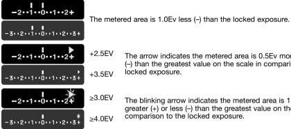
The arrow indicates the metered area is 0.5Ev more (+) or less (-) than the greatest value on the scale in comparison to the locked exposure.
