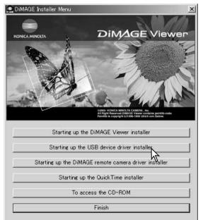
Before connecting the camera to the computer, place the DiMAGE Viewer CD-ROM in the CD-ROM drive. The DiMAGE installer menu should automatically activate. To automatically install the Windows 98 USB driver, click on the starting-up-the-USB-device-driverinstaller button. A window appears to confirm that the driver should be installed; click "Yes" to continue.
