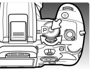
Program exposure is set with the exposure-mode dial (p. 39). Like full-auto program, program controls both the shutter speed and aperture required for each exposure. The operation is the same as described in the basic recording operation section on page 28. However, unlike full-auto program, functions set in this mode do not reset when the position of the exposure-mode dial is changed.
