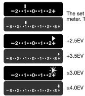
The set exposure is 1.0Ev less (-) than the exposure determined by the meter. The monitor scale is uses the manual metering (M.M.) indicator.
