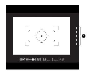
The spot AF area and local focus areas are illuminated briefly to indicate the point of focus when the focus is locked.
