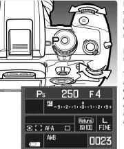
Program-shift function allows adjustment to the shutterspeed/aperture combination determined by the camera in both the program and full-auto program exposure modes. The built-in flash cannot be used with program shift. If the flash is raised, any changes made with program shift are canceled.
