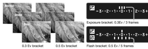
To make a flash bracket, raise the camera flash; the ambient exposure is not bracketed. The flash recharges between exposures. Exposure brackets are made when the flash is down.
