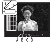
Press the shutter release button partway down to activate the autofocus and autoexposure systems (1). The viewfinder focus signal (A) confirms focus and the spot or local AF area (B) is illuminated briefly to indicate the point of focus. If the focus signal blinks, repeat the procedure.
