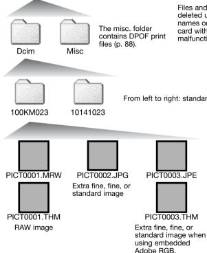
Files and folders on the memory card can be deleted using the computer. Changing file names or adding other types of data to the card with a computer may cause the camera to malfunction.
