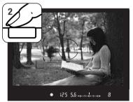
Without lifting your finger from the shutter-release button, recompose the subject within the viewfinder. Press the shutter-release button all the way down to take the picture.
