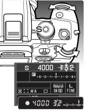
Shutter priority is set with the exposure-mode dial (p. 39). The photographer selects the shutter speed and the camera sets the appropriate aperture to ensure correct exposure.
