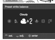
The rear control dial and the up/down controller keys adjust the white balance in seven levels: +3 to -3 (+4 to -2 for fluorescent). Except for fluorescent, the change of one unit is approximately equal to a 10 mired shift.
