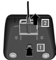
If you need to disconnect the plug from the charging cradle, press the release button **1** and disconnect the plug **2**.
