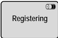
The handset registers automatically. Registration can take **up to 5 minutes**. **Do not remove the handset from the base station during this time.**
