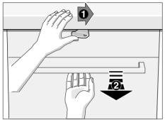
To open the door, move lever to right and pull door handle.
