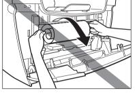
Do not pull the jammed paper upward; the toner on the paper will stain the machine and cause a permanent reduction in print quality.
