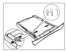
Make sure the paper stack does not exceed the load limit mark (A) and it is loaded under the hooks (B) on the paper guides.
