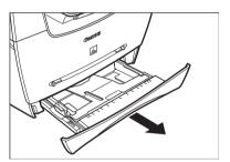
While holding the lock release lever on the paper guide at the rear of the cassette, slide the paper guide to the mark indicating the desired paper size.
