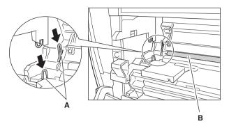
When removing the jammed paper, do not touch the transfer roller as its surface is very delicate and susceptible to finger oil and scratches, which may lead to print deterioration.
