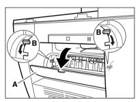
4 Hold both sides of the jammed paper and carefully move it inward, then gently pull it out.
