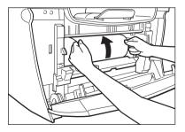
Foll the leading end of the paper outwards so that the printed surface is on the inside of the roll, then gently pull the rolled up paper out of the machine.
