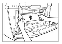
6 If the leading edge of the paper is visible but has not entered the imaging area, pull the paper forwards and roll it inwards.
