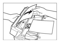
Widen the document guides until they stop, and remove the paper so as not to be caught by the guides. Open the ADF and gently remove the jammed paper from the ADF.
