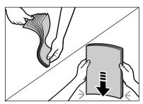
4 Load the paper stack in the cassette with the print side down.
