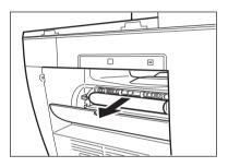
8 Carefully pull the jammed paper straight out through the rollers.
