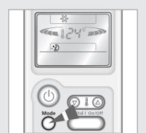
The Sleep Timer can be used when you are cooling or heating your room to switch the air conditioner off automatically after a period of six hours.
