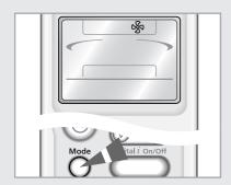
2 If the % is not displayed at the top of the remote control, press the  $\bigcap^{\text{\tiny{Mode}}}$  button on the remote control one or more times until it appears.
