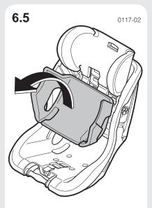
If the child's body weight exceeds 8 kg, the factory-fitted pelvic insert should be removed. This is located on the surface of the seat beneath the seat cover.
