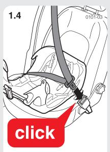
Pass the car seat belt over the top of the base unit and secure the belt in the buckle.
