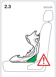
Insert the base unit into the car seat as illustrated. Position the reboard wedge (green) as shown.
