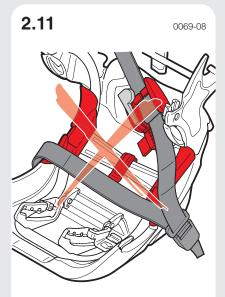
The car safety belt must be threaded through **all three** belt guides.
