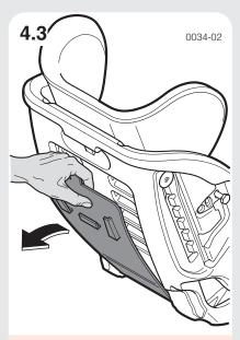
To adjust the shoulder belt positions, the seat shell must be removed from the base unit (see 1.1 and 1.2)!
