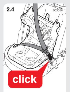
Pass the car seat belt over the top of the base unit and secure the belt in the buckle.
