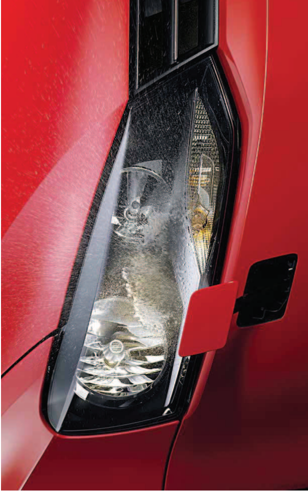
Headlight washers form part of the Winter pack , helping to improve safety in rain, snow and poor road conditions. Heated front seats provide comfort during cold weather, while heated windscreen washer jets help ensure visibility is maintained in the Winter months. Optional on all models.
