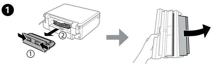
Pull out the rear cover and carefully remove the jammed paper.
