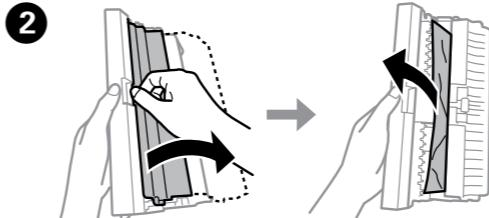
Open the rear cover and carefully remove the jammed paper.
