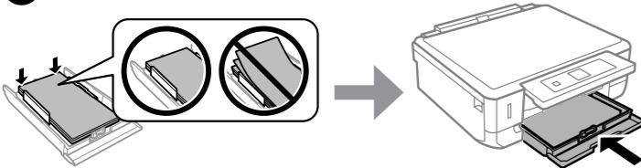
Align the edge guides to the edges of the paper. Keep the cassette flat and insert it back into the printer carefully and slowly.
