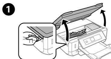
Open the scanner unit and remove all of the paper inside, including any torn pieces.
