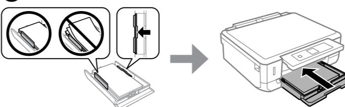
Slide the edge guides to the edges of the paper. Keep the cassette flat and insert it back into the printer carefully and slowly.
