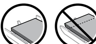
Load paper toward the edge guide with printable side face-down, and check that the paper is not sticking out from the end of the cassette.
