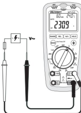
The mV-AC measuring range can only be selected via manual measuring range selection ("RANGE" button).
