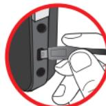
! When using a PC to charge the battery, do not power on the camcorder, or the charge will stop.
