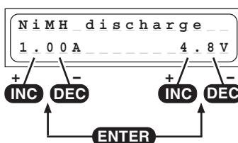
The typical purpose of this program is to determine the residual capacity of a transmitter, receiver or drive battery, or to discharge the pack to a defined level.
