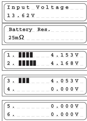
The current input voltage and battery resistance can be called up at any time by pressing the INC and DEC buttons **simultaneously**.
