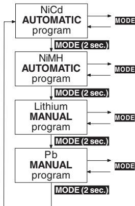
In the interests of clarity, the charge and set-up facilities of the charger are divided into four logical program groups. A separate program group is provided for each of the different battery types: **Nickel-Cadmium**, **Nickel-Metal-Hydride**, **Lithium-Ion / Lithium-Polymer / LiFePO<sub>4</sub> (LiFe)** and **Pb** (lead-acid) batteries.
