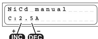
Select this program when you simply wish to recharge a battery using the set charge current.
