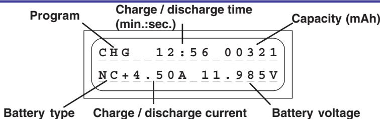
The two-line liquid-crystal screen displays in a clear form the important information generated during the charge / discharge process. The information remains visible on-screen until you disconnect the battery that is being charged. Once you connect another battery for charging, the previously displayed values are erased, and cannot be called up again.
