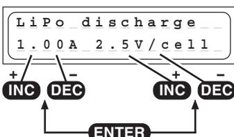
The purpose of this program is to determine the residual capacity of a Lithium pack which has not been fully discharged.
