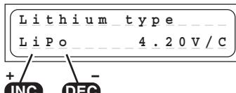
(LiPo, Lilo or LiFe) affects the charge termination voltage. If you find that a Lithium battery has unexpectedly been charged only to the 2/3 full mark, you have probably set the incorrect battery type at this point. **Caution:** if you set an incorrect value at this point, the battery may be damaged irreparably, and could even explode!
