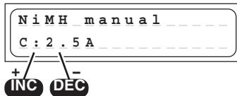
Select this program when you simply wish to recharge a battery using the set charge current. You can adjust the charge current using the INC / DEC buttons, but only **before** you connect the pack for charging. The range available is 0.1 A to 5.0 A.
