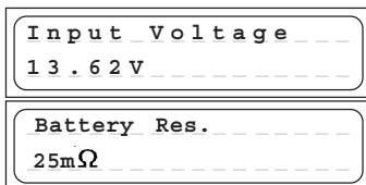
The current input voltage and battery resistance can be called up at any time by pressing the INC and DEC buttons **simultaneously**.
