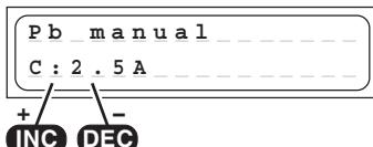
In this program you can set the maximum permissible charge current using the INC / DEC buttons, but only before you connect the lead-acid battery for charging. This setting only determines the top limit which the charger is permitted to feed to the battery.
