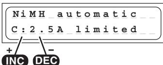
In this program the charger detects the type of Ni-MH battery connected to it, and adjusts the charge current accordingly to avoid overcharging the pack.
