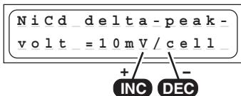
The automatic charge termination circuit (battery full detection) works on the proven Delta Peak principle (also known as the Delta-V process), which is already in use in millions of chargers.
