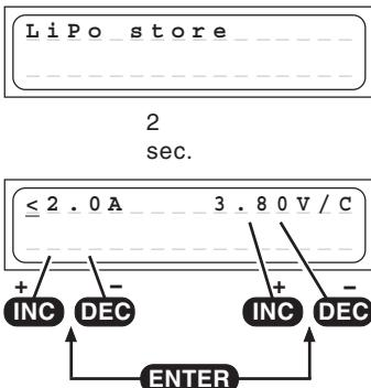
This program does charge or discharge the battery to the best storage voltage.
