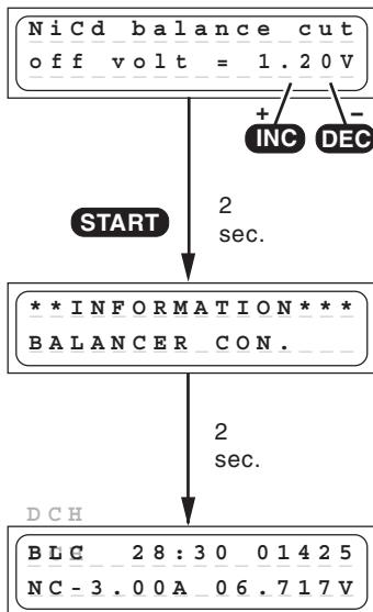
The discharge balancing program does discharge and balance up to 6 cells of a battery pack.
