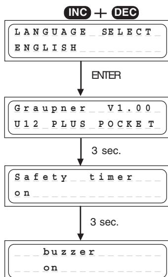
Press and hold the INC and DEC buttons simultaneously, then switch on the charger to get the language selection display. Select your language using the INC or DEC button and confirm with pressing the ENTER button.
