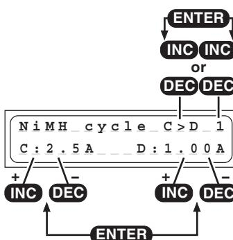
This program is designed to optimise the capacity of a battery, and balance the state of its cells.
