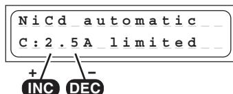
In this program the charger detects the type of Ni-Cd battery connected to it, and adjusts the charge current accordingly to avoid overcharging the pack.
