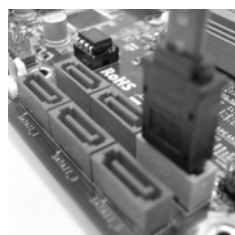
Connect the SATA data cable to the orange SATAII connector (SATAII_6)
